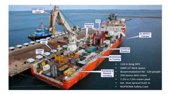
The project also used the Sapura Intervention Compensation System (ICS) which provides compensated guidewires/podlines and compensated sheaves over the moonpool to allow safe deployment of umbilical's and wireline tools during vessel heave. The ICS has two independent H-frames, each with two in-line compensation systems providing up to 6 tonnes of guide wire compensation and is mobilized onto the vessel in just two lifts.
